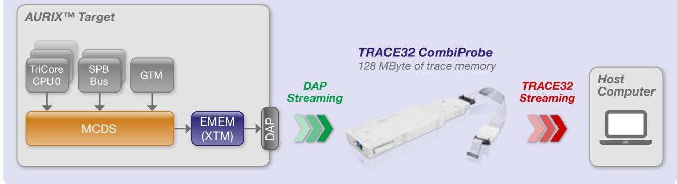
Lauterbach has been supplying its new CombiProbe TriCore DAP for the AURIX™ family from Infineon since October 2016. This means TRACE32 now offers comprehensive run-time analyses for all AURIX users whose target hardware does not provide an AGBT interface.
